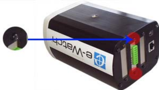
Figure 2-6 Camera Back with Cover Plate Screws Highlighted
