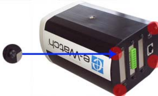
Figure 2-7 Camera Back with Back Cover Screws Highlighted
