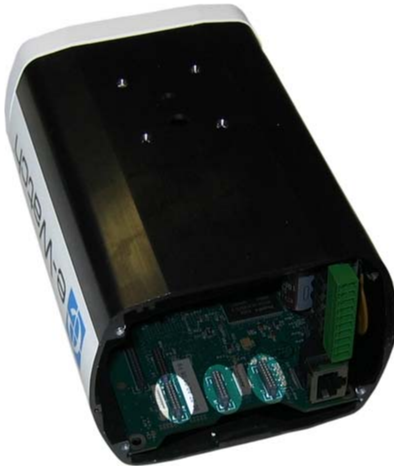
Figure 2-5 Open Camera with possible connectors
